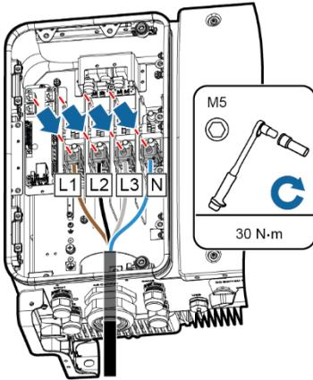
d. Five-core cable (including the ground cable and neutral wire)
