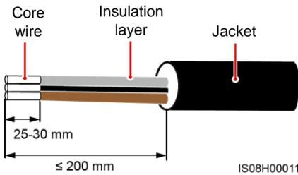
b. Four-core cable (including the ground cable but excluding the neutral wire)
