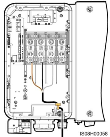
5. Tighten the thread-lock sealing nut and seal the waterproof connector.
