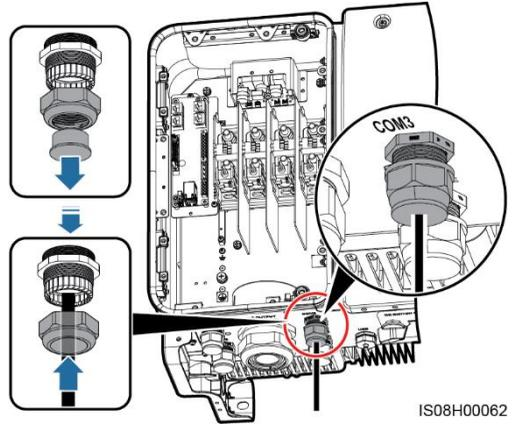
3. Loosen the minus screw on the cable connector, and connect the solar tracker power cable.
