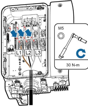
b. Four-core cable (including the ground cable but excluding the neutral wire)
