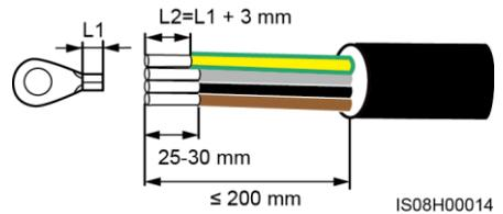
c. Four-core cable (excluding the ground cable but including the neutral wire)
