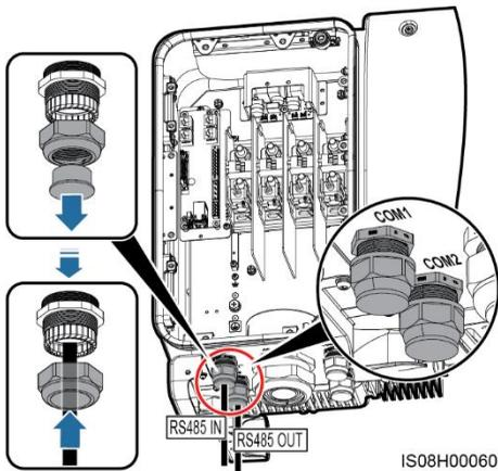
3. Remove the cable terminal base from the terminal block. Connect the communications cable to the terminal base.
