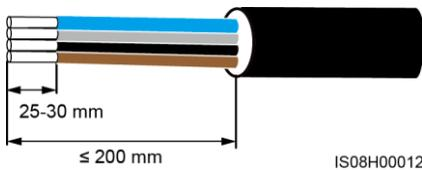
d. Five-core cable (including the ground cable and neutral wire)
